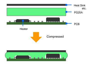
PG25A is the lowest modulus type of Putty Type available. Ideally suited for applications requiring low compression force on the component. It offers the high performance that very easily conforms in and around protrusions and depressions on components to make complete, reliable physical contact.
